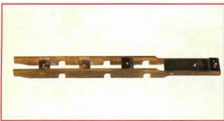
Above: Although it does not look like much at first glance, this is actually a Canadian National 4-6-0 brass frame constructed from simple brass shapes, which were screwed and soldered together.
